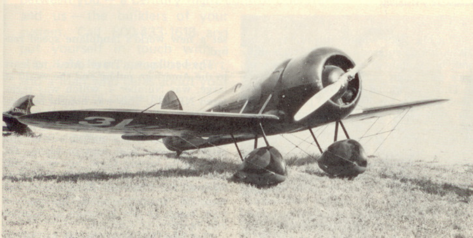
This view shows the new NACA cowling and wheel plants of the Travel Air Mystery Ship R614K as well as its unique wire bracing system.
