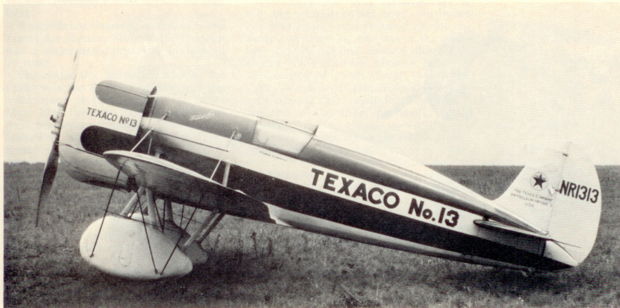
Frank Hawks' NR1313 featured a modified cockpit. After takeoff, he lowered his seat and then slid the windshield aft to form a drag-reducing roof. Side panels provided the necessary visibility.
